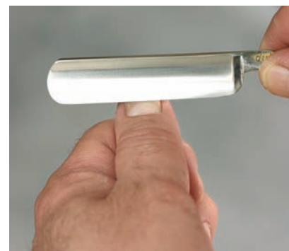
Figure 6-46 Testing a honed razor.
